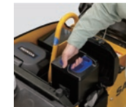
"eGX" and "Honda Mobile Power Pack e:" equipped SAKAI HEAVY INDUSTRIES, LTD. Electric Walk- Behind Roller "HV620 evo"
