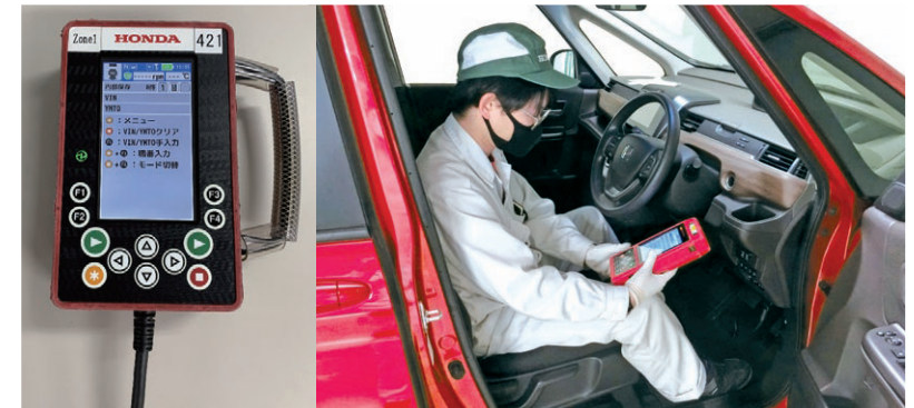
Inspection using the LET system
