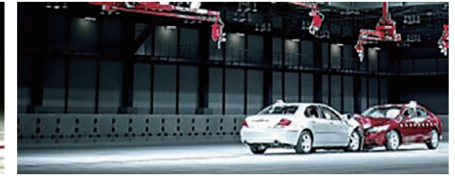
Indoor omnidirectional crash test facility
