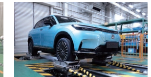
Bench vibration test Actual vehicle vibrations are reproduced on a testing bench together with analyzing issues.
