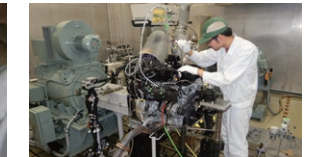
Testing engine functionality and performance The functionality and performance of assembled engines are verified on a bench.
